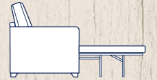
2/3 SEATER SOFABED (Low feet only) Two fold slatted and webbed metal action. Depth open 2280mm
